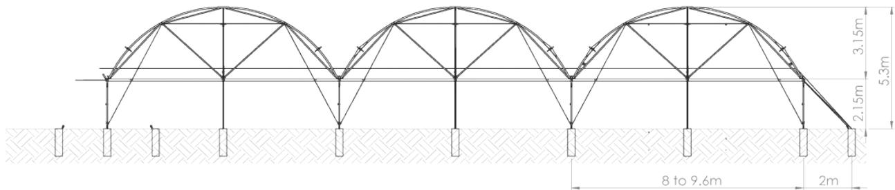
Agrotem's Hybrid Model is a high-strength upgraded multi-tunnel, bright structure with birdproof roof ventilation and optional rain gutters. This is our unique model, offering excellent cost to value for berries and herbs growers.
