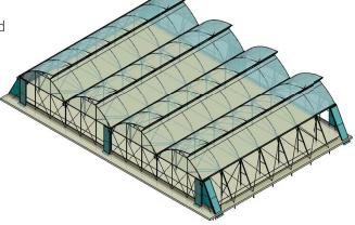
The size of this model is 9.6m wide and the Raingutter height is 4.5m.
