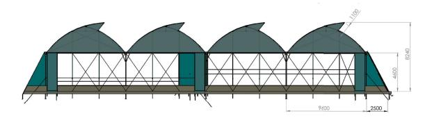
Agrotem's Marissa Model is a Polyethylene cover structure of the fixed top-vent type. It is Reinforced for regional weather condition, and includes side curtain and slide doors. It offers excellent cost to value for flowers and vegetables growers.
