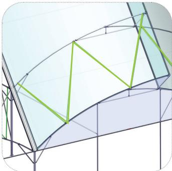
**Diagonal pipes support / reinforcement (between first to second arch)** - reduces installation, maintenance time and costs.
