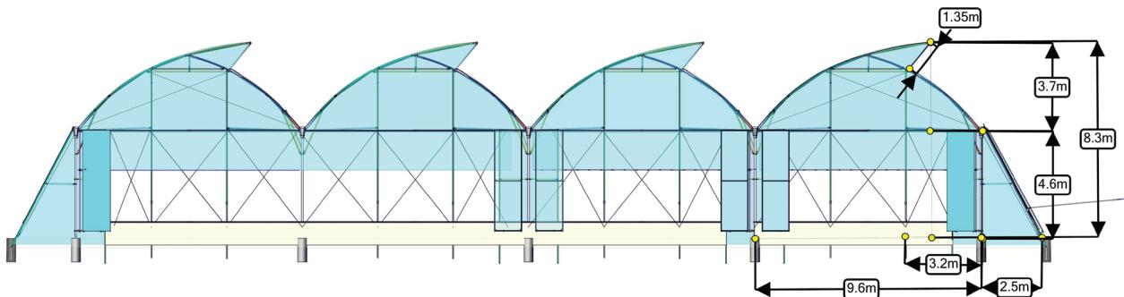
Agrotem's Marissa Model is a Polyethylene cover structure of the fixed top-vent type. It is Reinforced for regional weather condition, and includes side curtain and slide doors. It offers excellent cost to value for flowers and vegetables growers.
