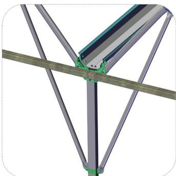
**Pipes support / reinforcement between column to arch**
