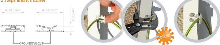
Tool recommended: Standard multigrip plier L250mm with self gripping teeth and locking button
